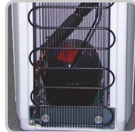
Hermetically sealed reciprocating compressor
