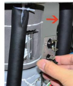
2. There is enough heat transfer paste on the tank and the old thermostat to simply wipe the face of the replacement thermostat against the old one. (Figure 4-7-7).
