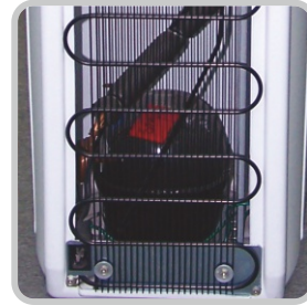
Hermetically sealed reciprocating compressor
